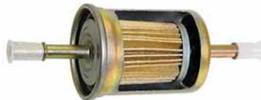
Clean filters protect the fuel system components and help to increase gas mileage.
