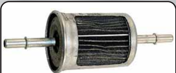
Dirty filters can cause drivability problems, reduce fuel system component life & increase fuel consumption.
