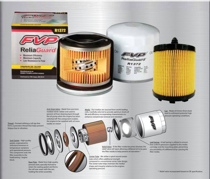
All FVP ReliaGuard Oil Filters are designed to trap maximum contaminants to protect vital engine components. High baked filter media ensures maximum filtration and unrestricted oil flow.
